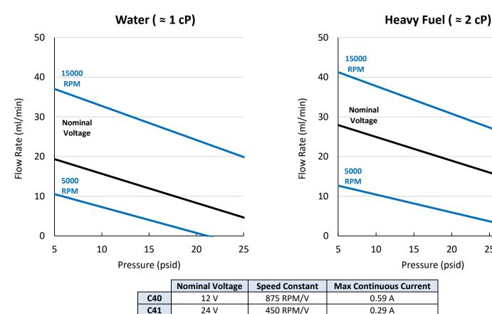
176 RPM/V NOTES: Dashed lines indicate intermittent operation; speed constant may vary at higher pressures; RPM flow lines indicate performance at typical maximum and minimum speeds;
